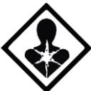
Do not inhale air/Hydrogen mixture that exceeds 4% (by volume) and ensure Hydroxy gas has been adequately scrubbed (see manual for details) prior to inhalation
