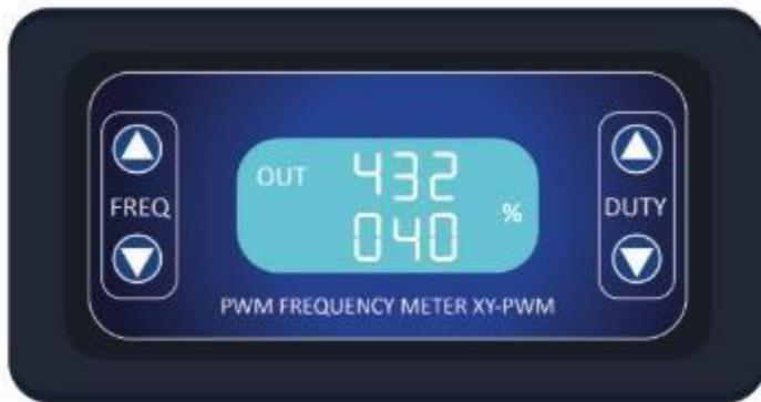
The Duty Cycle is the time during each period (pulse of FREQ) that the electricity is on and can be adjusted using the DUTY buttons. If the Duty Cycle % is set for 30 that means the electricity is on for 30% of the time and off for 70% of the time.
