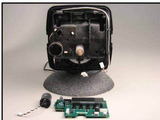
Unhinge the drive bracket by using the two finger tabs on the top left and top right of the black drive bracket – then thread the power cable into the valve and attach to the connection marked 12 VAC on the green PC board.
